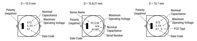
Displays nominal capacitance, maximum operating voltage serial number, polarity, etc.
