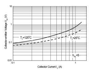
Collector-emitter Saturation Voltage
