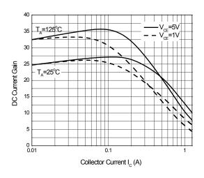
DC Current Gain vs. Collector Current
