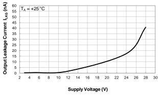
**Output Leakage Current vs Supply Voltage**
