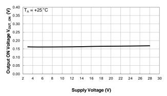
Output ON Voltage vs Supply Voltage
