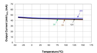
Output Current Limit vs Temperature
