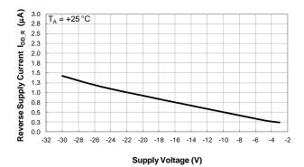
Reverse Supply Current vs Supply Voltage
