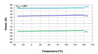
Switch Points Bop and Brp vs Temperature
