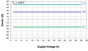
Switch Points Bop and Brp vs Supply Voltage
