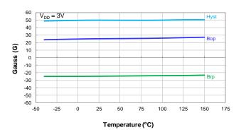
Switch Points Bop and Brp vs Temperature
