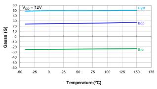
Switch Points Bop and Brp vs Temperature
