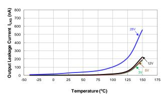
**Output Leakage Current vs Temperature**
