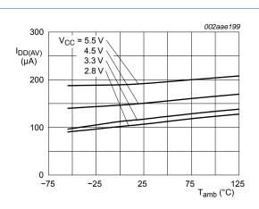
Fig 15. Average supply current versus temperature; I<sup>2</sup>C-bus active
