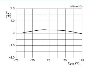
Fig 19. Typical temperature accuracy versus temperature;  $V_{CC} = 3.3 \text{ V}$
