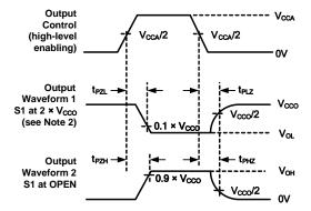
Figure 6. Voltage Waveforms Enable And Disable
