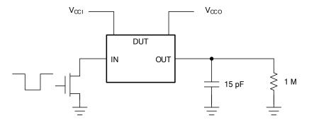
Figure 2. Data Rate, Pulse Duration, Propagation Delay, Output Rise And Fall Time Measurement Using An Open-Drain Driver
