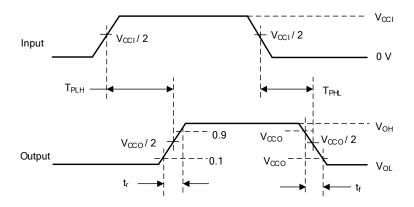
Figure 5. Voltage Waveforms Propagation Delay Times
