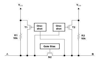
Figure 7. Architecture of a RS0102 Cell
